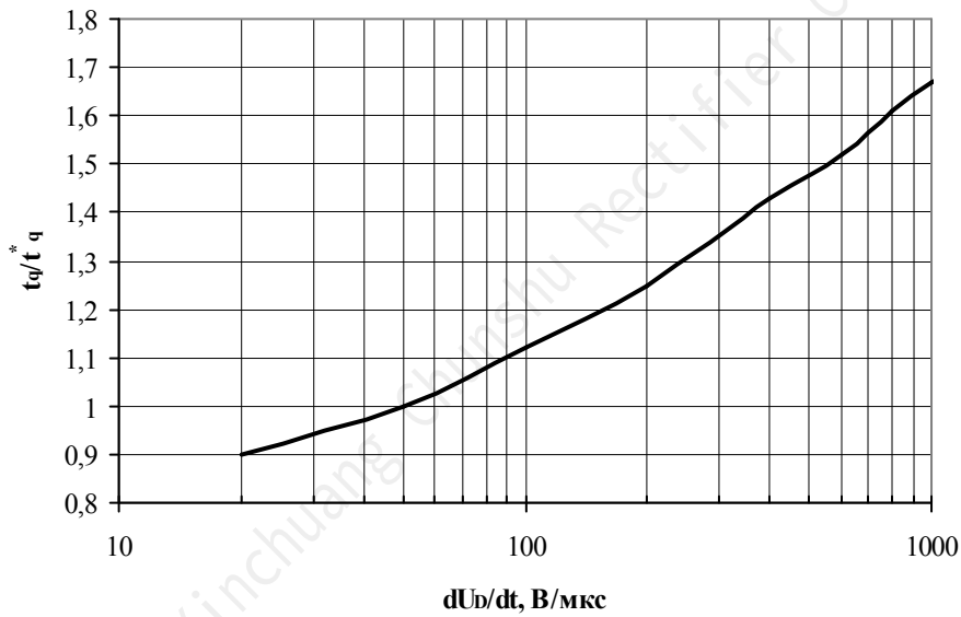
Fig. 30 Turn-on time t_q vs. rate of rise of off-state voltage (di_T/dt)_f .
