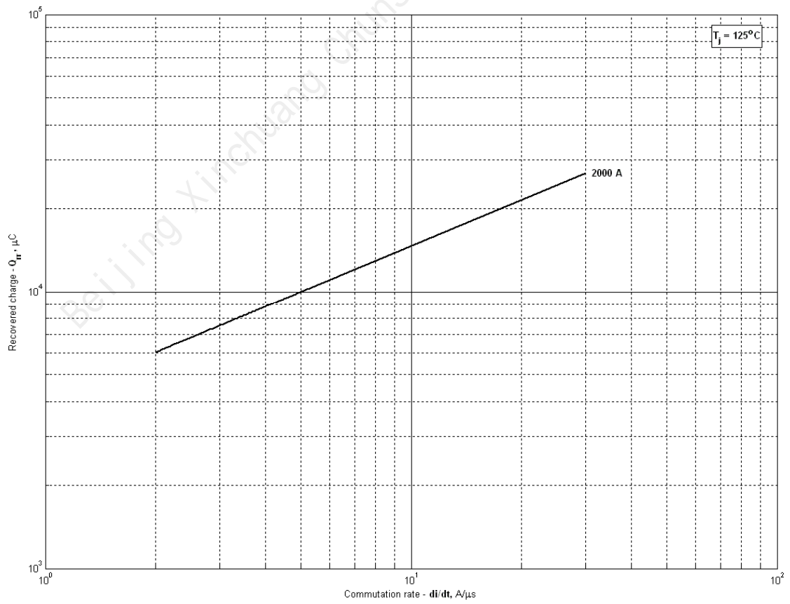
Fig 6 - Recovered charge, Q_{rr} (linear)
