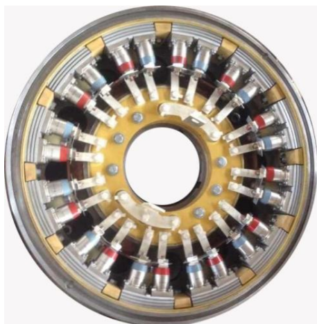
Rectifying Disc for 85MW Generator
